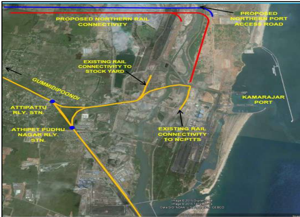
Figure - 1.7. External Rail Road Connectivity to Kamarajar Port
